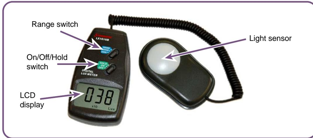
When measuring light intensity (or illuminance) in an office or classroom environment, we need to place the light meter on the **working plane**, which in this case is the level of the desks or worktops.
